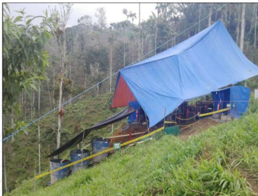
Figure 3. Water used to cool and lubricate the core bit and the drill string gravitates through settling tanks to remove suspended mud before being recycled in the drill hole.
