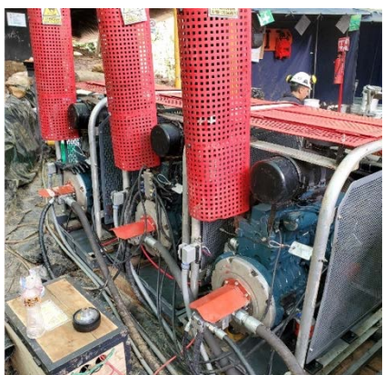
Figure 4. Small diesel motors are combined in series to provide the hydraulic power required by the drill rig.
