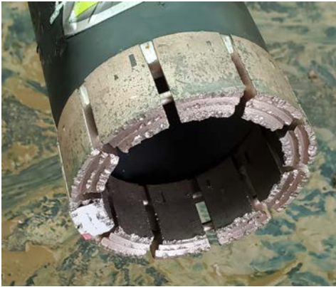
Figure 2. A drill bit is the diamond-encrusted tungsten steel ring that rotates to cut the rock. The cylinder of rock core gradually moves up the center of the core bit as the bit moves down through the rock.
