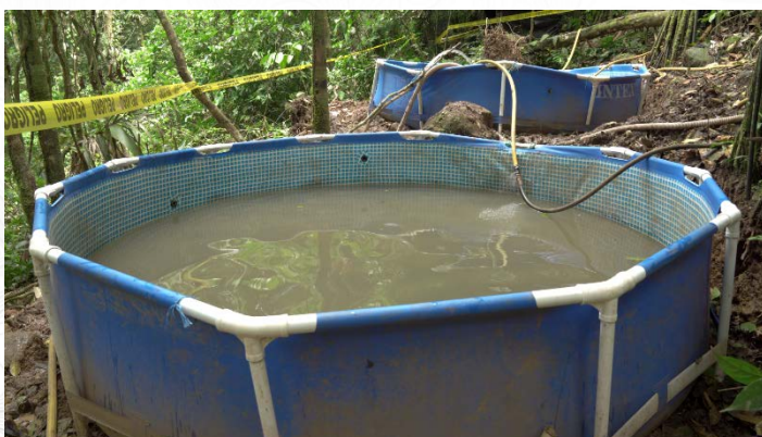
Figure 5. Rain water is collected in large collapsible tanks that can be drained and moved from one drill site to the next.
