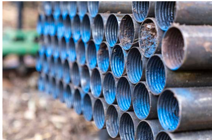
Figure 1. Threaded steel tubes – drill rods – stacked, ready to be attached, one by one as the hole deepens, forming the drill string that transfers the torque of the drill rig to the diamond bit.
