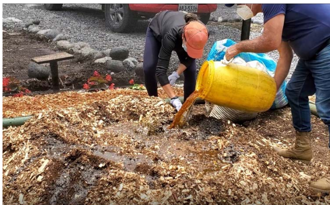
Figure 10. Bio-treatment of waste oil from the drilling and exploration camps. The oil and grease is poured into a mixture of equal quantities of chicken manure, coarse sawdust and topsoil, is moistened with water, and left to
