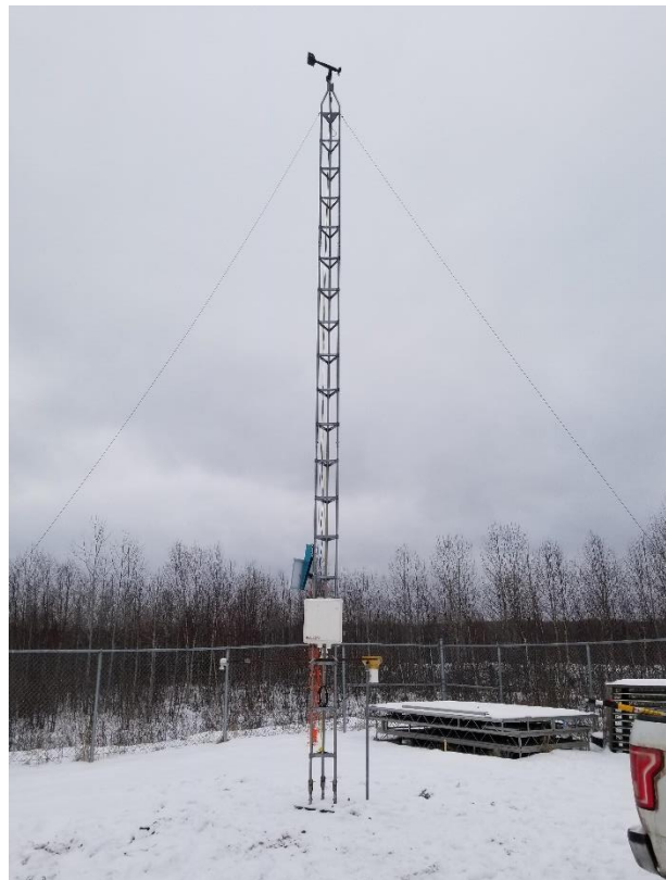
Photograph 1: View of meteorology station used to measure and record temperatures, wind direction and speed, humidity, barometric pressure and precipitation.
