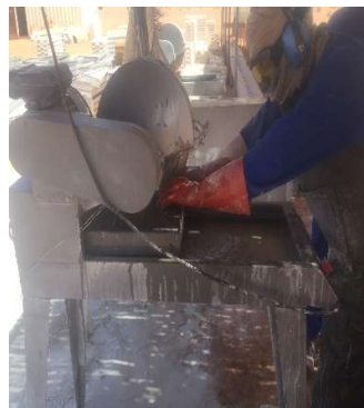
Fig 2 Water sprayer cut down the dust
