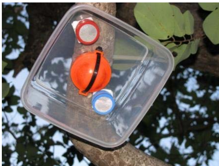
Plate 5.6 Radon Samplers Deployed for Passive Monitoring
