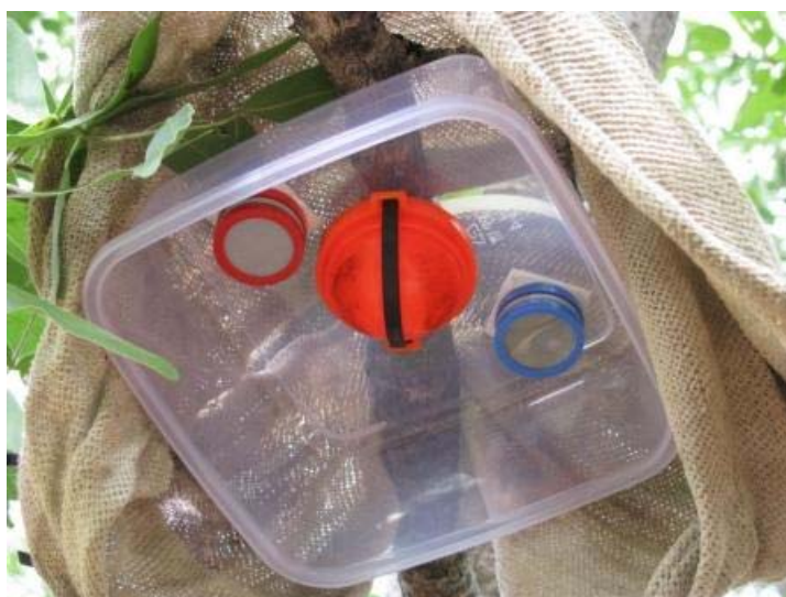
Plate 5.5 Layout of NO 2 and SO 2 Passive Samplers
